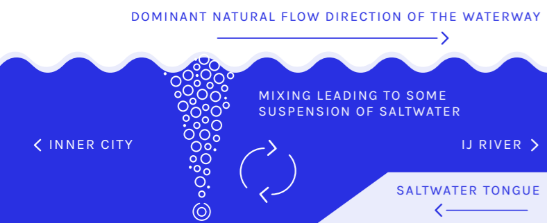
Figure 1: Hypothesis for saltwater dynamics around Bubble Barrier Amsterdam.
